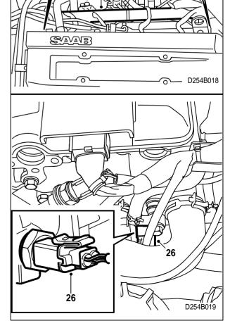
26 Plug the connector into the temperature sensor.
