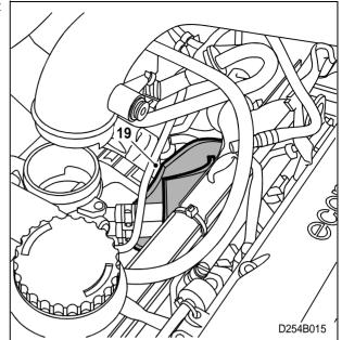
20 Install the crankcase ventilation hose in so that the check valve is located above the coolant hoses. The crankcase ventilation hose must follow the route of the lower coolant hose through the intake manifold and then on to the oil trap.
