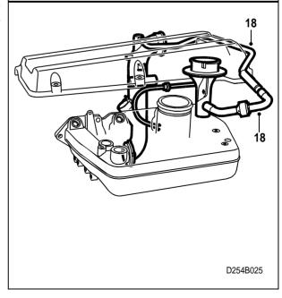
19 Install the insulation under the throttle body coolant hose so that the insulation's short sides point upward.
