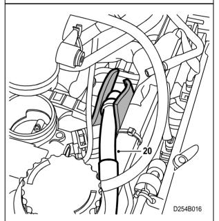
21 Connect the oil trap's upper hoses. If the hose with part no. 55 560 463 is replaced then the nipple enclosed with the hose must not be used. Use the nipple enclosed with the spare parts kit.
