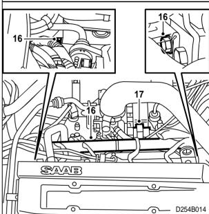
18 Connect the new hose kit (with T-connection) between the nipple on the oil filler pipe and the connection on the turbo's intake manifold.
